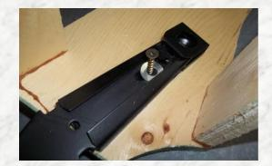
4-Install the screw and washer in the hole of the metal bracket.
